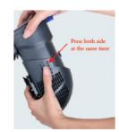
Step 3 Referring to the picture, use your fingers to press the release button, pull the bottom unit to separate the top and bottom units.
