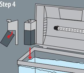
First read the Aqua-Flow filter manual. Install the AquaFlow filter into the aquarium. Your aquarium filter helps to keep the water healthy therefore you need to clean it weekly. Click the cartridge from the filter and rinse it with fresh tap water. The cartridge contains active filter carbon that absorbs harmful substances from the water therefore you need to replace the cartridge monthly.
